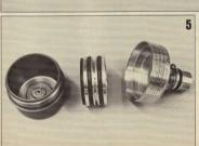
4 The dissected lower chamber. The piston is in the fork tube (arrow), the spring on the damper rod is to prevent topping. The two seals retain damping oil and air pressure. The ridged aluminum sliders on the 125 are 10% lighter than previous ones.
